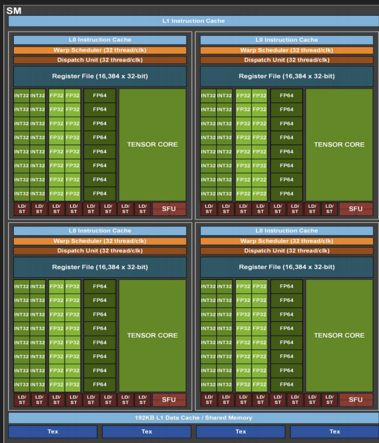
NVIDIA GA100 Architecture (just for DGX and servers)
